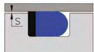
Sealing gap limited by a back-up ring
