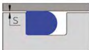
O-ring under pressure in normal working condition
