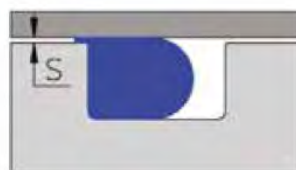
O-ring extruded into sealing gap
